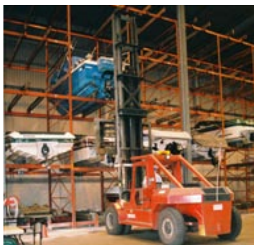
The heavy equipment operators at the East Chicago Marina use forklift trucks to haul boats carefully onto the dry stack.
