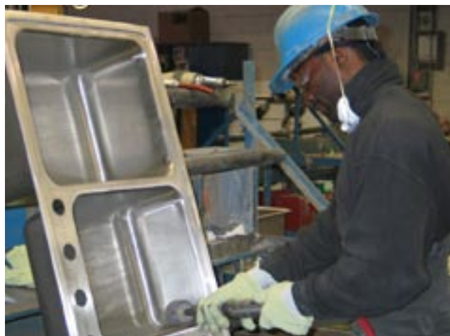
Sanders polishes a sink bowl to a shine at his job at Elkay Manufacturing.
